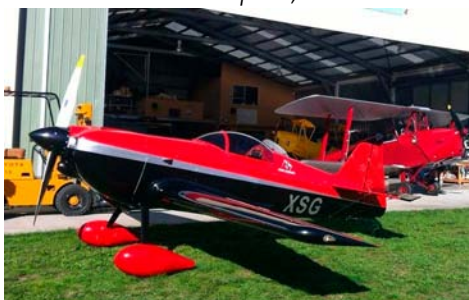
DR-107 One Design built from 'nature's composite'.
