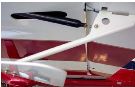
Aileron Spades to lighten control forces.
