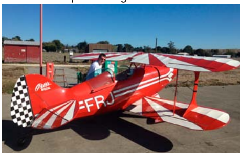
Top and bottom ailerons on the Pitts Special.
